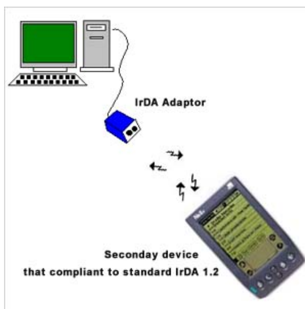
Figure 6.2: IrDA point to point link (from: http://www.sixca.com/eng/articles/irda )
